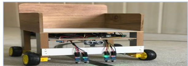
Figure 9: The ARW line while traveling using IR sensors.
