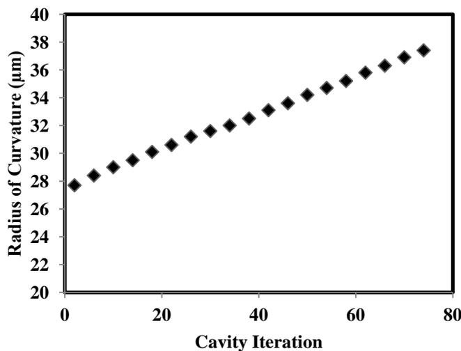
Fig. (6): Variation of radius of curvature with cavity iteration.
