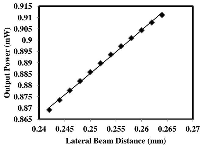
Fig. (5): Variation of lateral beam distance with output power inside the resonator.
