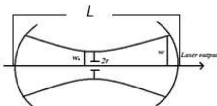
**Fig. (1):** Represents a typical low power gas laser resonator
