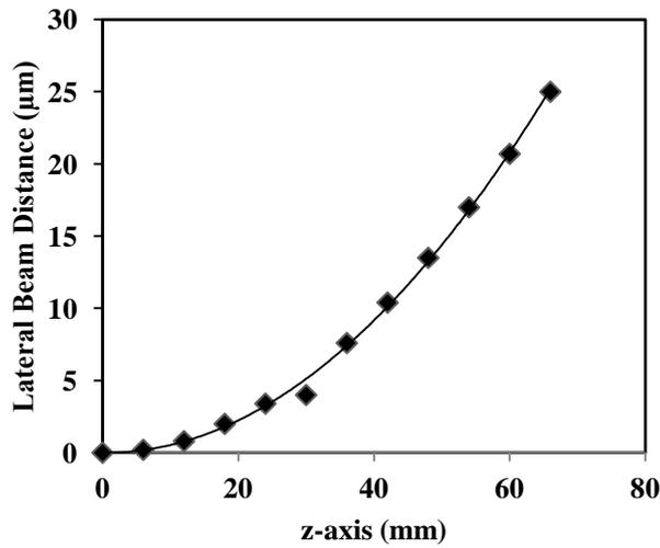
Fig. (4): Variation of lateral beam radius with distance along z-axis
