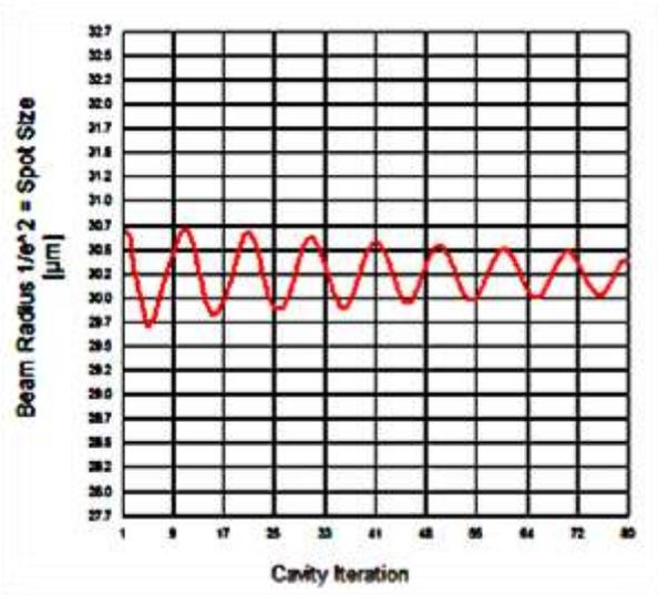
Fig. (2): Variation of the spot size versus cavity iteration.
