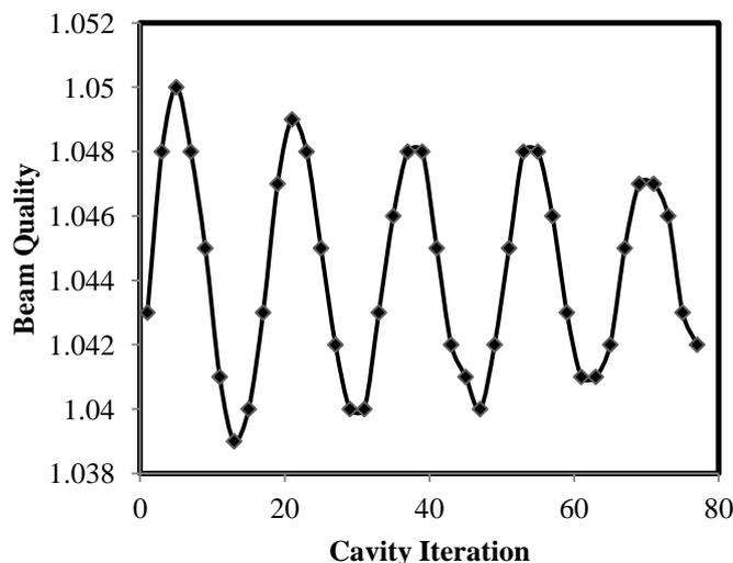
Fig. (7): variation of beam quality with cavity iteration.
