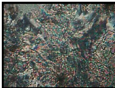
Figure 4: Texture of S_mC phase for 0.5 mole fraction of CNBMeOA at 86°C (magnification 250)
