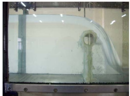
Fig.(2): Side view of flow over weir
