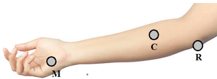
Figure 1. Figure showing electrode placement. The AC current (20 μA) provided by the instrumentation is applied to the skin through the M electrode
