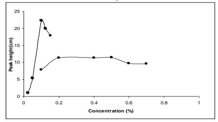
Figure (7): Effect of the concentration of reagents on peak height (•) p-toluidine (■) p-nitroaniline
